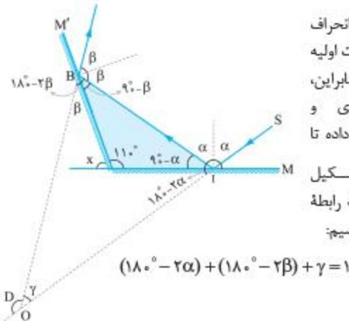
$$D = 180^\circ - \gamma = 180^\circ - 40^\circ = 140^\circ$$
